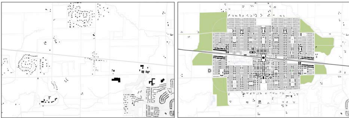
FIGURE 10: LaFox, Illinois existing conditions (left); LaFox, Illinois 2100 build-out plan (right), with constructed wetlands local passive wastewater treatment fields at perimeter.
